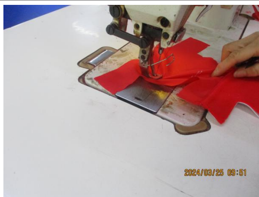
Needle guard for sewing machine.JPG
